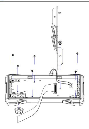
6. Remove the keypad circuit board assembly.
