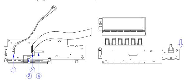
9. Remove all the 9 screws affixed to the power supply board using the T10 Torx screwdriver. Separate the power supply board carefully from the main body of the generator in order to avoid being scratched by the sharp metal edge.
