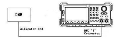
3. Select a 10 kHz Sine waveform of the generator and set the amplitude to the values listed below in sequence.
