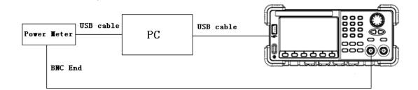
3. Select Sine waveform of the generator and set the amplitude to 0.5 Vpp and frequency to the values listed below in sequence.
