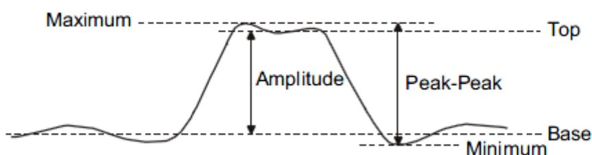
Figure 86 Voltage Measurements
