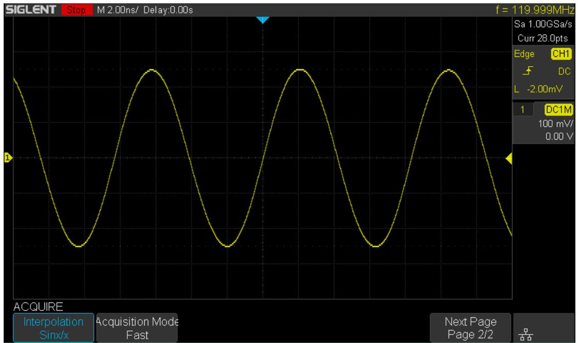
Figure 20 Sinx/x Interpolation
