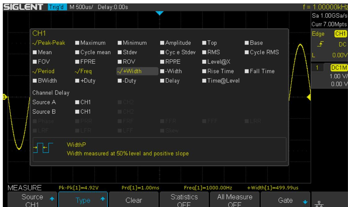
Figure 90 Select the Measurement Parameter
