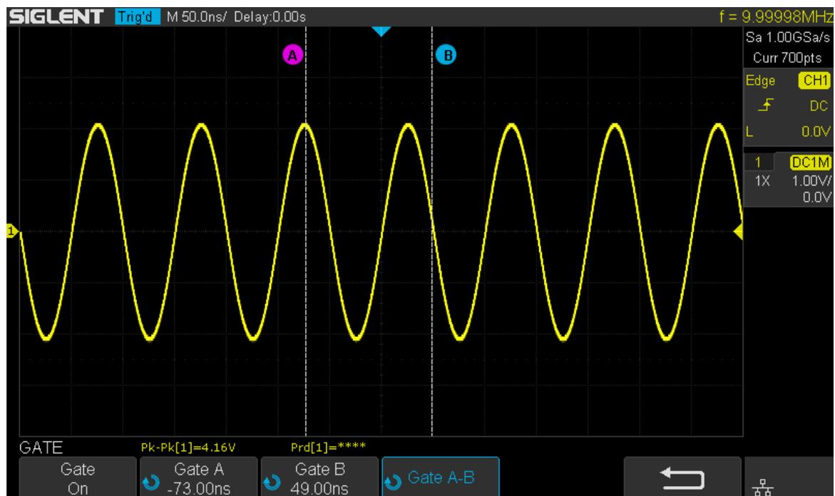
Figure 93 Gate Measurement
