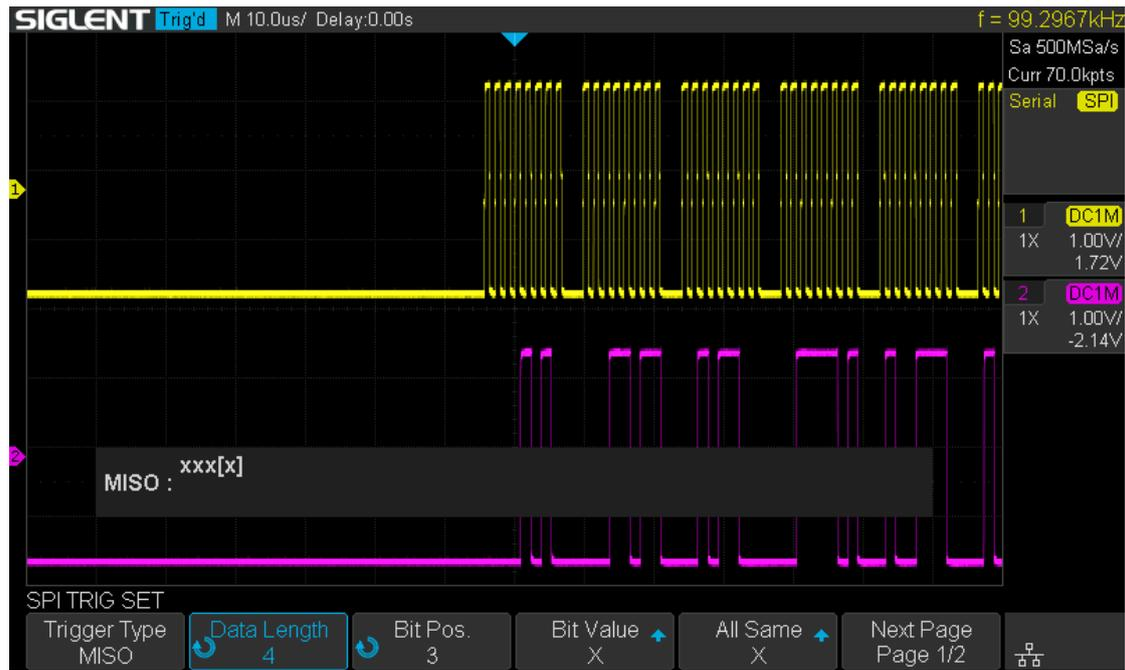
If the data width is set to be greater than 8 bits (such as 16 bits), the clock idle time between 8-bit data packets T2, and then set the timeout time to a value between  $T1/2+T2$  and  $T3$ .
