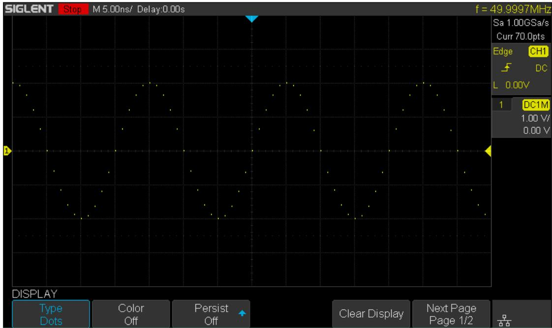
Figure 95 Dots Display
