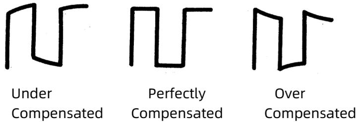
4. Use a nonmetallic driver to adjust the low-frequency compensation adjustment hole on the probe until the waveform displayed is as the “Perfectly compensated” in the figure above.
