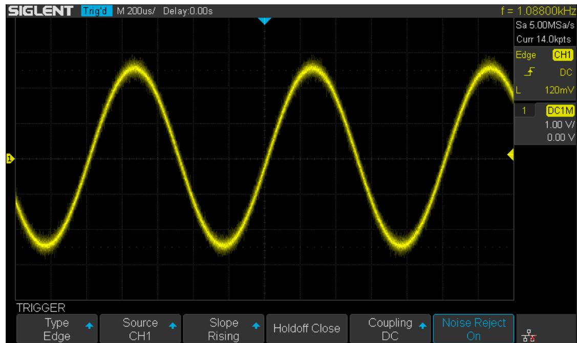
Figure 29 Turn on the Noise Reject
