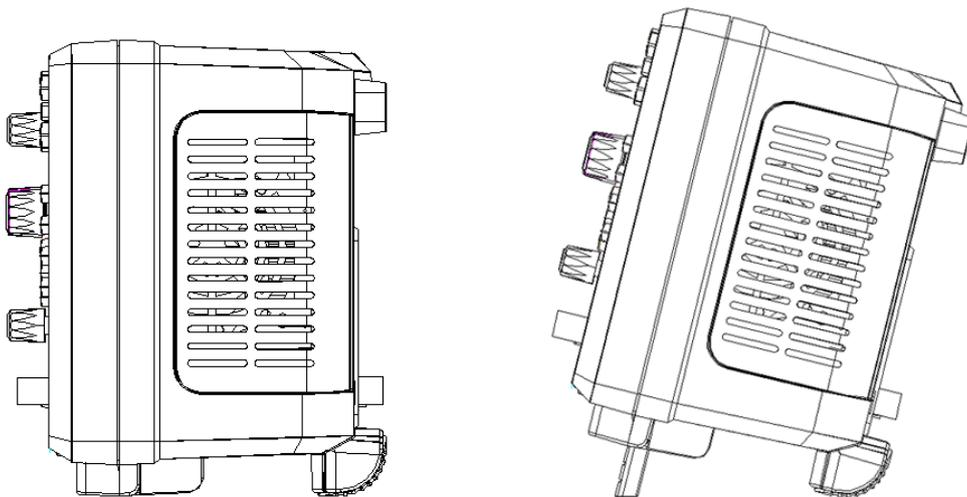
Figure 5 Adjust the Supporting Legs
