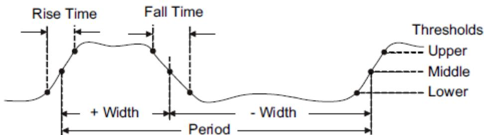
Figure 89 Time Measurements
