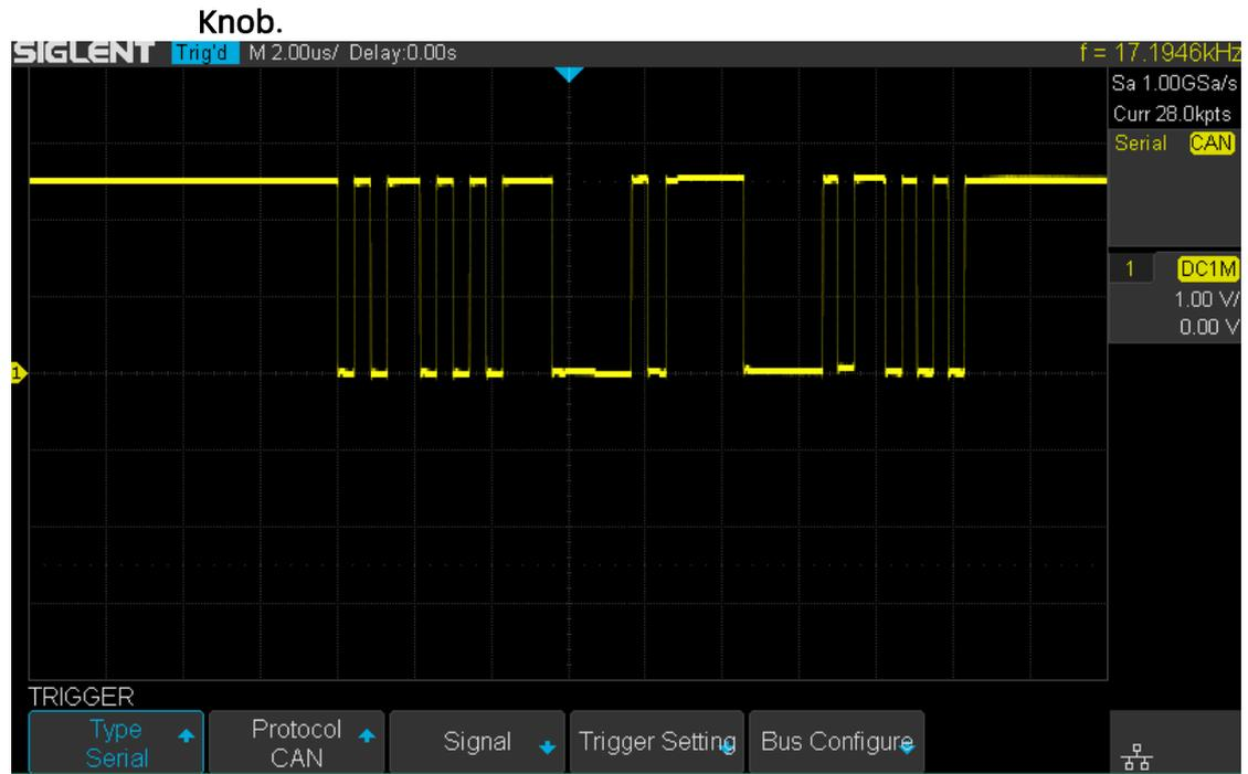
Figure 61 CAN Trigger
