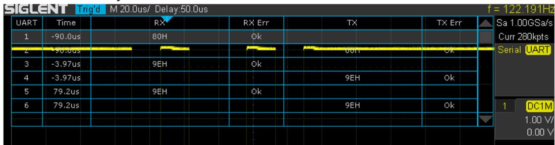
Figure 59 UART Decode List Display
