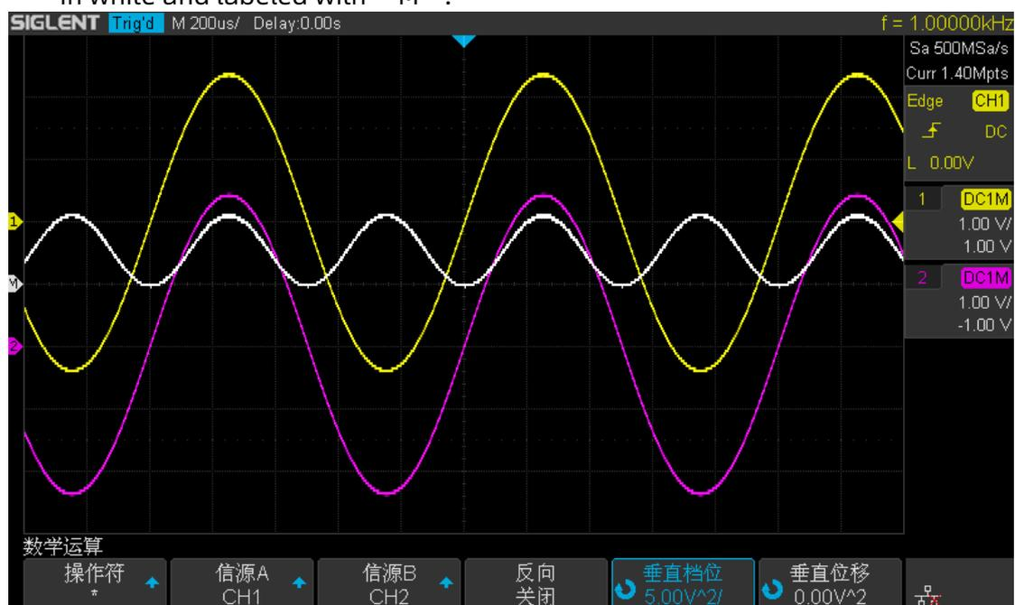
Figure 71 C1\*C2 Waveform
