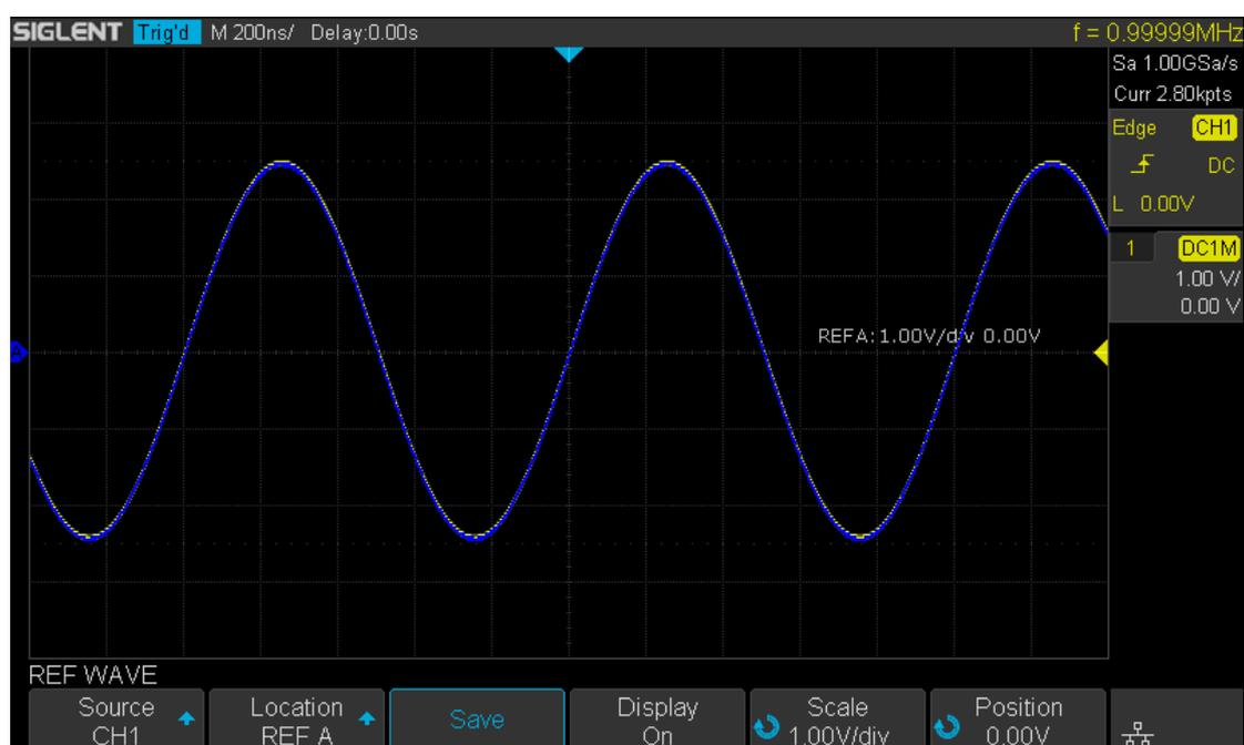
Figure 69 Reference Waveform
