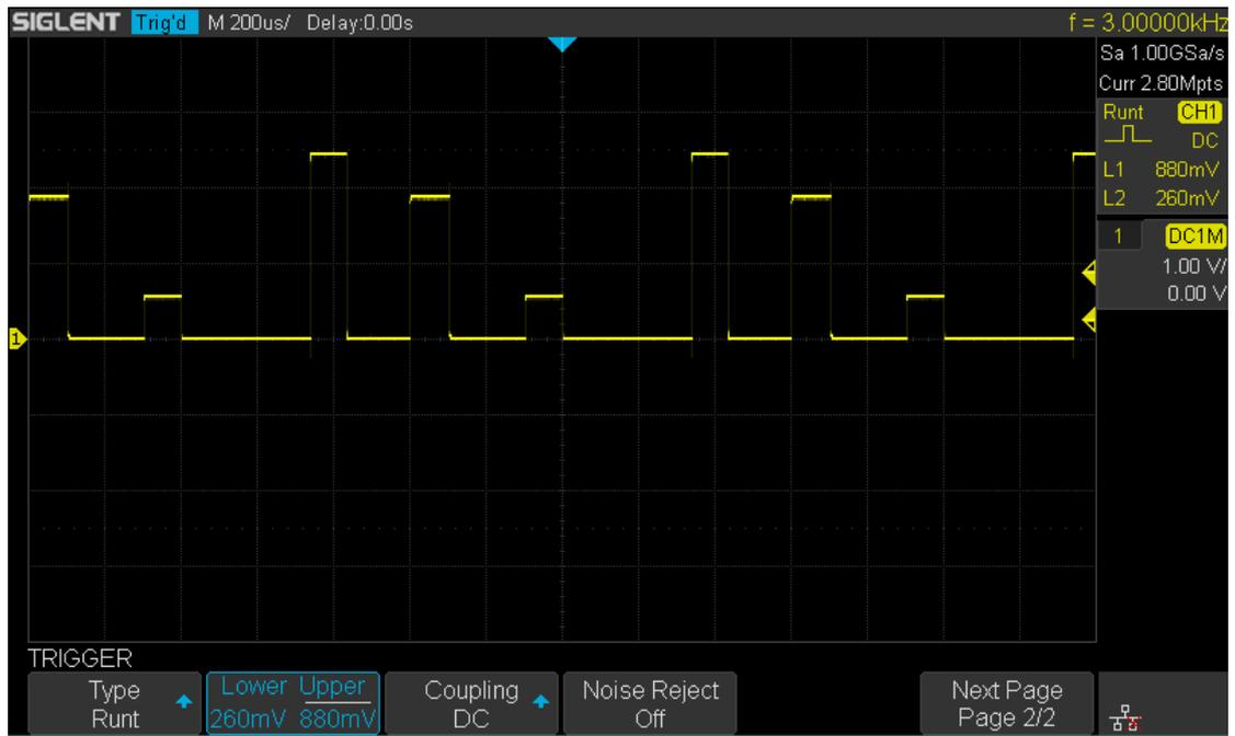
Figure 39 Runt Trigger
