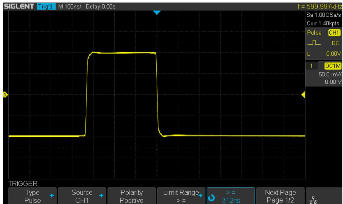
Figure 32 Pulse Trigger
