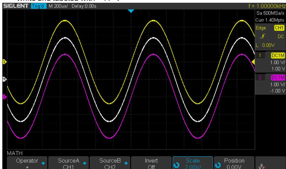
Figure 70 C1+C2 Waveform
