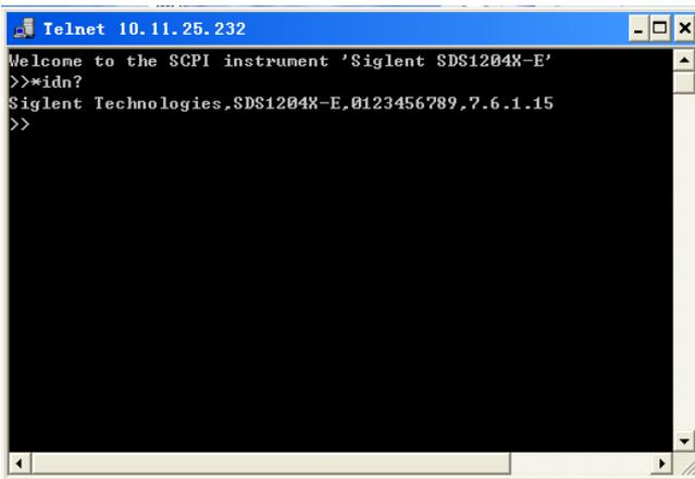
6. To exit the SCPI> session, press the Ctrl+] keys simultaneously.
