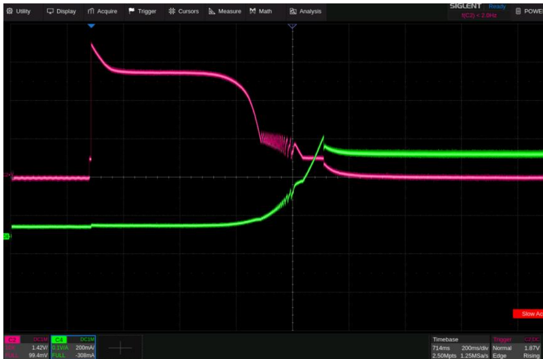
Figure 8 Voltage and Current Waveforms on MOSFET During Power-up
