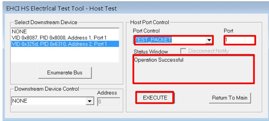
**Display Test Pattern:** Remove the USB device from the host port under test. Use a USB cable to connect the port under test to the test fixture (which is already connected to the oscilloscope). The oscilloscope will now display the test pattern.
