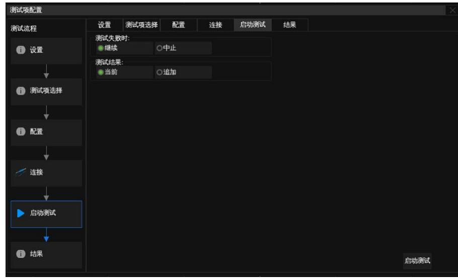
**3.5** Follow the pop-up prompts to complete the test. Upon completion of all test items, the test results will pop up. If multiple test items are selected in one round, a pop-up will 提示 (提示: prompt) the connection method for the next item when proceeding. It supports returning to the "Configuration" section mid-process to modify the signal source for that test item. After modification, click "Start Test" in the pop-up to continue testing.
