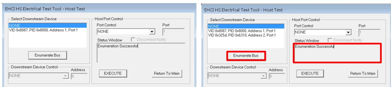
**Port Control:** In "Host Port Control," enter the host port number under test in "Port." The selection in the "Port Control" dropdown is related to the test item, e.g., select **【TEST\_PACKET】** for signal quality tests, **【SUSPEND】** for suspend and resume tests, **【TEST\_J】** for High-Z level tests. Click **【EXECUTE】**, and the status window should display "Operation Successful".
